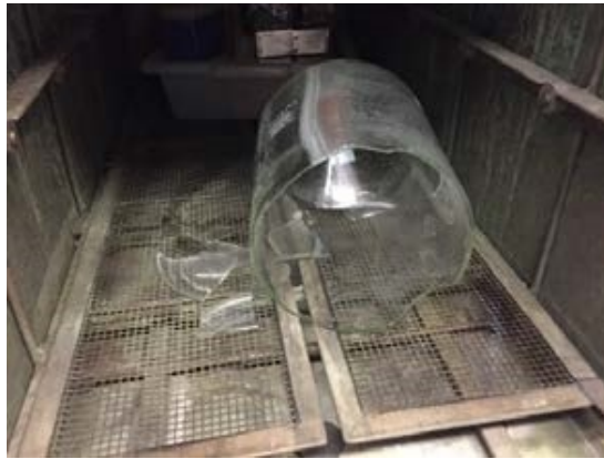
Burst bottle placed directly on autoclave rack.
