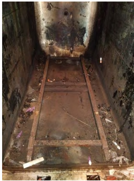
Liquid from biohazardous waste bags sprayed from an autoclave into a hallway at the University of North Carolina, Chapel Hill. A clogged drain/strainer was a partial cause (photos courtesy of UNC EHS).
